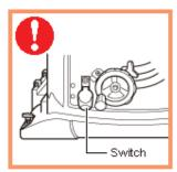
When starting the use of tool, make sure that the **SWITCH IS IN OFF POSITION** BEFORE CONNECTING THE PLUG.
