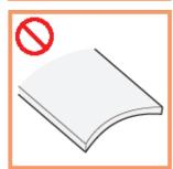
Do not rip workpiece that is twisted, warped or does not have a straightedge to guide it along the fence.
