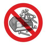
Remove any dust and debris from the battery, and keep it away from other metal objects (screws, nails, etc.).
