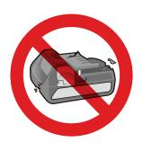
Do not pierce battery with a sharp object such as a nail, strike with a hammer, step on, throw or subject the battery to severe physical shock.
