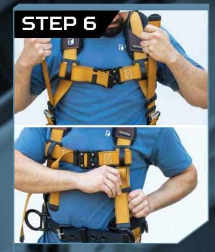
While standing up straight, adjust torso straps to your height and to remove slack.
