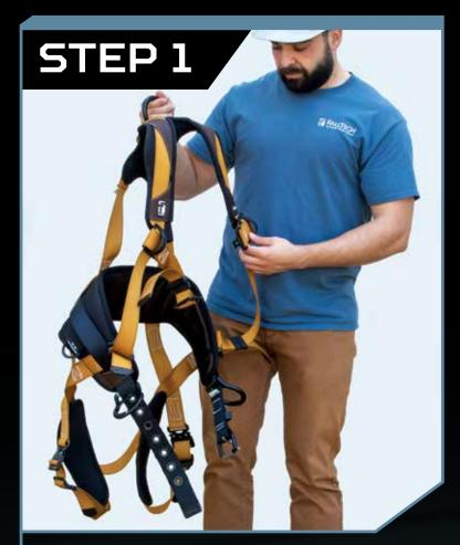
Holding the harness by the dorsal D-ring, shake it to allow all straps to hang freely and untwisted.
