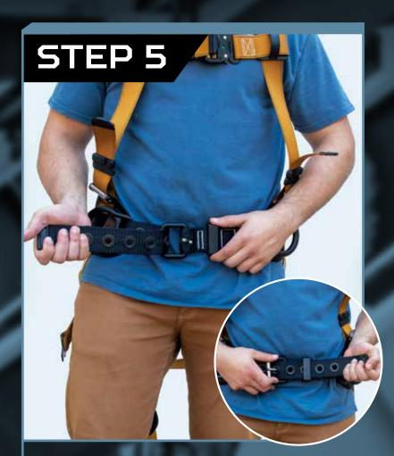
**Buckle the waist belt and secure the loose** end in the belt retaining keeper provided.
