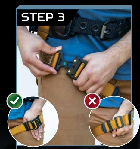
Pull leg straps up and between legs then connect to buckles located closest to each hip.
