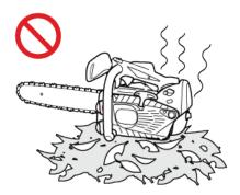
Once you have started the engine, do not put the tool on flammable materials such as dried grass.
