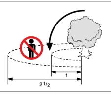
While cutting a standing tree, ensure that no other person is within a distance of 2 1/2 tree lengths from the tree.
