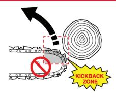
Do not hit the KICKBACK ZONE of the guide bar and saw chain on an object such as log or branch, otherwise the violent backward and/or upward motion of the chain saw guide bar may occurs unexpectedly and such motion (KICKBACK) can cause serious or fatal injury.
