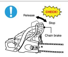
Check whether the CHAIN BRAKE (a device for stopping the chain) works properly before use.
