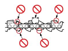
Do not use dull or damaged saw chain.
