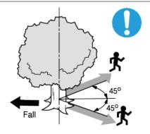
Before cutting a standing tree, ensure that there is no other person or obstacle in the falling direction.
