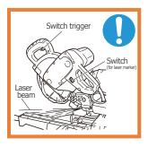
Make sure before plugging the power plug into the receptacle that the main body and the laser marker are turned off.
