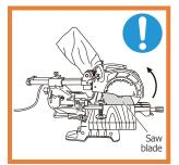
Always wait for the rotation of the blade to stop completely before lifting the saw blade.
