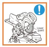
Always confirm that the lower guard is in the proper place before using the miter saw.
