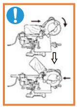
When slide cutting, never pull the handle toward the operator, since this could cause the saw blade to kick up from the workpiece.
