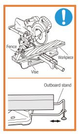
Always firmly clamp or vise to secure the workpiece to the fence; otherwise the workpiece might be thrust from the table and cause bodily harm.
