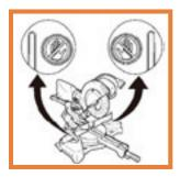
Never place your limbs inside of the line next to warning sign "or or "while the tool is being operated."
