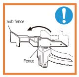
In the case of left bevel cutting, see the instruction manual and ensure that the saw blade does not contact the sub fence.
