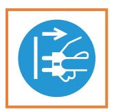
Make sure that the **PLUG IS DISCONNECTED** from the power source (or, for battery-operated tools, the battery is removed) when preparing for use or inspecting your tool.
