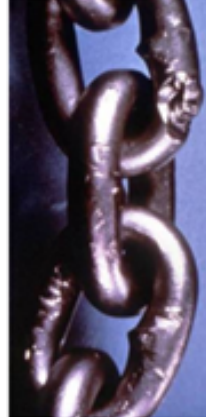
Heat Damage, Nicks & Gouges
